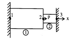
AluminumSteel $A1 = 2400 \text{ mm}^2$  $A2 = 600 \text{ mm}^2$  $E1 = 70 \times 10^9 \text{ N/m}^2$  $E2 = 200 \times 10^9 \text{ N/m}^2$
