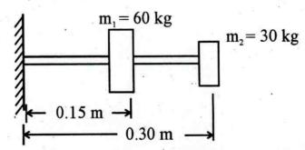
Take  $E = 2 \times 10^{11} \text{ N/m}^2$  and cross section moment of inertia of the beam  $I = 4 \times 10^{-7} \text{ m}$ .
