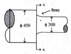
The shaft is machined by a turning process. The section x-x is subjected to a constant bending moment of 500kN-m, the shaft material has  $S_{ut} = 500MN/m^2$  &  $S_{yt} = 350MN/m^2$  and endurance limit in bending for 7.5mm diameter specimen of  $210 \, MN/m^2$ . Notch sensitivity is 0.8. Expected reliability is 90%. Determine life of shaft. Theoretical stress concentration factor can be taken from tabulated values.
