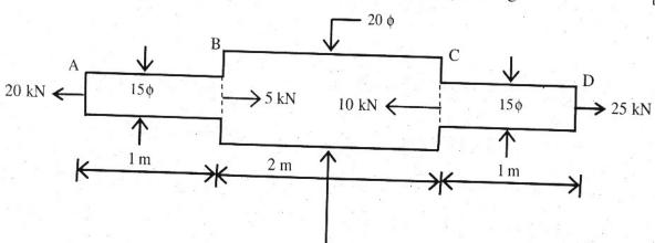
Diameter of portion AB, BC and CD are 15, 20 and 15 mm respectively. Find the elongation of bar. Take E = 200 GPa.
