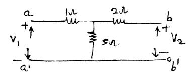
2. Derive the condition of reciprocity and symmetry in Z parameters
