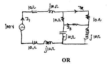
1. For the given network determine the transform impedance (8)
