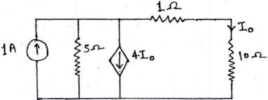
2. Find the current in the  $10\Omega$  resister in the circuit of given Figure using Thevenin's theorem. What is the power loss in that resister?
