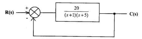
Determine the characteristics equation of the system,  $W_n$ ,  $\xi$ ,  $W_d$ ,  $t_p$ ,  $M_p$ , the time at which the first undershoot occurs, the time period of oscillations and the number of cycles completed before reaching the steady state. (12)
