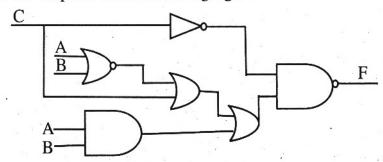
Q.5 Complete the truth table for the combinational circuit shown in the figure -
