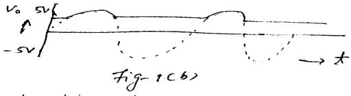
Assume the input wavefrom is  $v_i = 5\sin \omega t$
