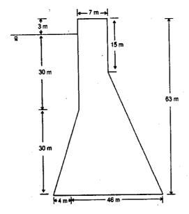
Check the stability of the gravity dam shown above for the reservoir empty and reservoir full conditions. Calculate the principal stresses and shear stress at toe and heel of the dam. Consider only self weight, weight of water, water pressure and uplift pressures. Average shear strength (q) = 1.4 MPa and Wc = 24 KN/m3.
