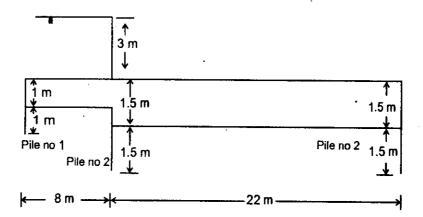
Calculate uplift pressures at key points of all the three piles of the structure shown above. Also check the thickness provided and the exit gradient. The safe exit gradient is 1.5
