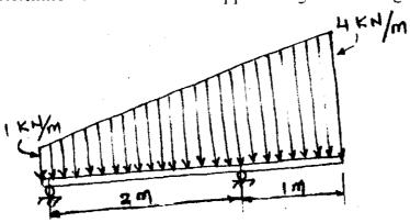
b) Determine Reaction value at the roller support B and C using virtual v method.
